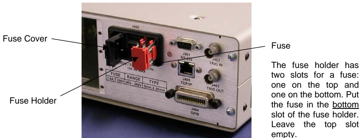
Figure 2-1, Changing Fuse for Main AC Power
