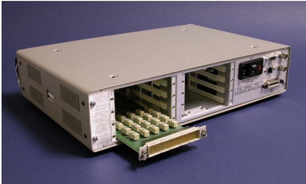
Figure 2-2, Inserting a Plug-In
